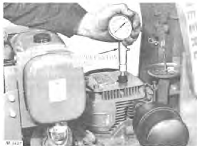
Fig. 8-Testing Engine Compression
