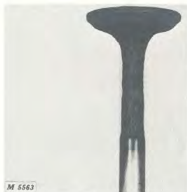
Fig. 3 - Valve Stem Corrosion
