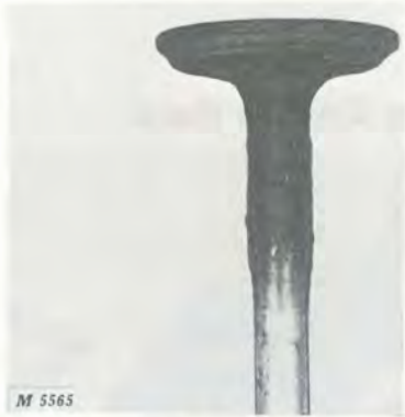
Fig. 5 - Gummy Valve Causing Valve to Stick
