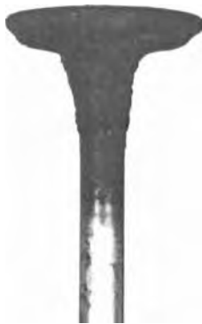
Fig. 2-Lead Deposits on Leaky Intake Valve
